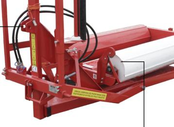
The ribs on the bale wrapper drums improve their durability and prevent sliding of the bale.
